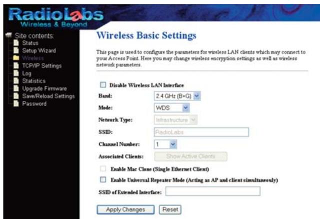
On the left-side menu, click on Wireless, and then WDS Settings. WDS must be set to Enable. If it is not, check the box for Enable WDS
