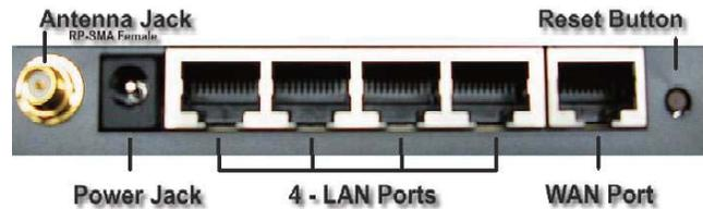
Plug power into the O2Link Router, use an RJ-45 (cat5) Ethernet cable to connect to the LAN port of the router to your PC's Ethernet port. You will use this to configure the settings of the Router.
