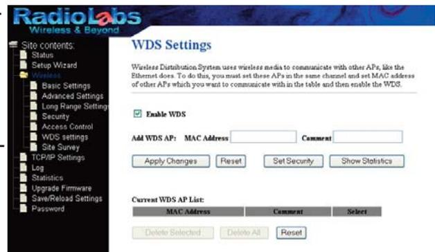
Press Apply Changes when done. The Router will reboot, and when the screen refreshes, the Access Point's MAC address will be listed under the Current WDS List
