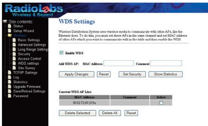
Your wireless bridge is invisible, and cannot be detected by wireless devices. But to further secure your bridge you may now set the bridge with Encryption. Starting with the O2Point Access Point, in the web based configuration, select WDS Settings then Select the “Set Security tab.”
