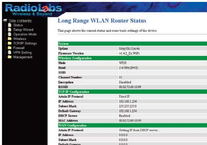
on the left side menu, and then select Basic Settings. Set the Mode to WDS. Change the Wireless Channel from Auto to a channel 1-11 you choose. Make a note of the channel that you've chosen, because the other end of the bridge will need to be on the same channel. **DO NOT** Enable Universal Repeater Mode (Acting as AP and client simultaneously). Click Apply Changes. Your Router will reboot in 30-60 seconds (keep an eye on the WiFi light when it starts blinking again your Router or AP is reset).
