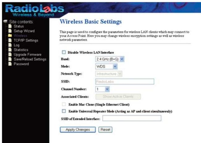
Now the O2Link's IP Address is 192.168.1.2, enter that into the Address Field at the top of your web browser and hit enter. Now click on the Wireless tab, and select Basic Settings. Change the wireless channel to match the one you set for the first O2Link. Also make sure the Mode is set to WDS. Click Apply. Your O2Link will reboot in 30-60 seconds.
