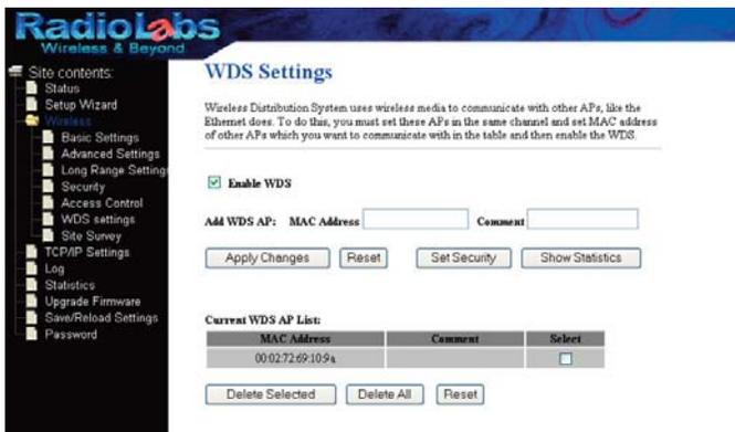
Just to recap what we have done: On the Bridge Kit (two O2Link Routers) under “Wireless” then “Basic Settings” we changed the Operation Mode to WDS and set a Channel. Then under “WDS Settings” we have swapped LAN Mac Addresses between the two units.
