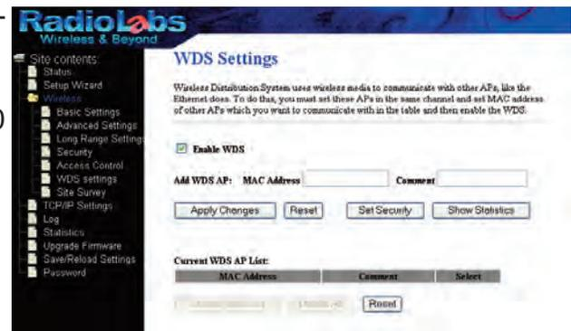
Press Apply Changes when done. The GS1000 will reboot, and when the screen refreshes, the second GS1000's MAC address will be listed under the Current WDS List
