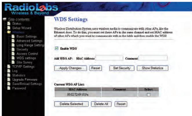
Your wireless bridge is invisible, and cannot be detected by wireless devices. But to further secure your bridge you may now set the bridge with Encryption. In the web based configuration, select WDS Settings then Select the “Set Security tab.”
