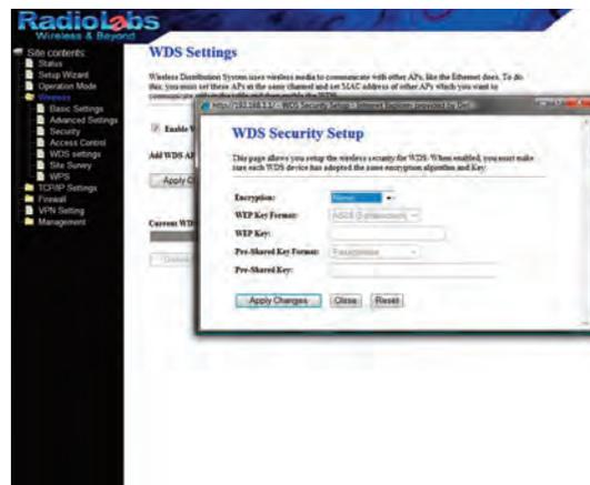
Below is an example of setting WEP security settings. Change wireless encryption from “none” to “WEP”. WEP keys may be any of 4 different types choose one of the following types by selecting the “Set WEP Key” button:
