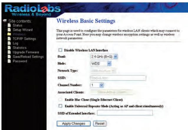
On the left-side menu, click on Wireless, and then WDS Settings. WDS must be set to Enable. If it is not, check the box for Enable WDS
