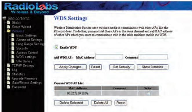
The two GS1000 Bridge units are now linked by a wireless bridge. Open your browser and enter the first GS1000's IP address in the address bar (192.168.1.1) You now should be able to access the Web-Based Configuration Utility of the first GS1000 wirelessly via the Second GS1000. If you have an
