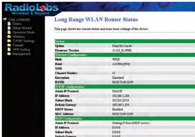
left side menu, and then select Basic Settings. Set the Mode to WDS. Change the Wireless Channel from Auto to a channel 1-11 you choose. Make a note of the channel that you've chosen, because the other end of the bridge will need to be on the same channel. **DO NOT** Enable Universal Repeater Mode (Acting as AP and client simultaneously). Click Apply Changes. Your GS1000 will reboot in 30-60 seconds (keep an eye on the WiFi light when it starts blinking again your GS1000 is reset).
