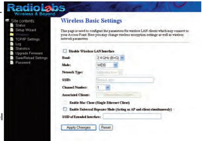
Now the GS1000's IP Address is 192.168.1.2, enter that into the Address Field at the top of your web browser and hit enter. Now click on the Wireless tab, and select Basic Settings. Change the wireless channel to match the one you set for the first GS1000. Also make sure the Mode is set to WDS. Click Apply. Your GS1000 will reboot in 30-60 seconds.
