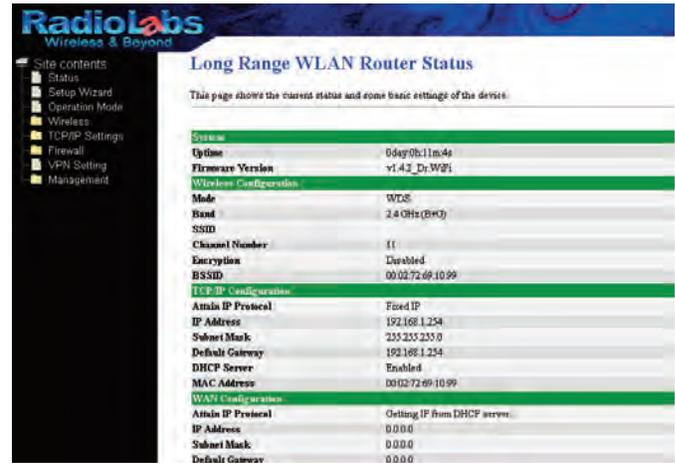
In the Web-Based Configuration Utility, click TCP/IP then LAN, in the IP Address field change the IP address to 192.168.1.2 and Disable the DHCP. Click Apply. Your GS1000 will reboot in 30-60 seconds.
