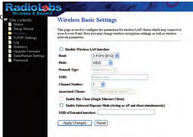
In the Web-Based Configuration Utility, click on the Wireless tab, and select Basic Settings. Change the wireless channel to match the one you set for the O2Link Router. Also make sure the Mode is set to WDS. Click Apply. Your O2Point Access Point will reboot in 30-60 seconds.
