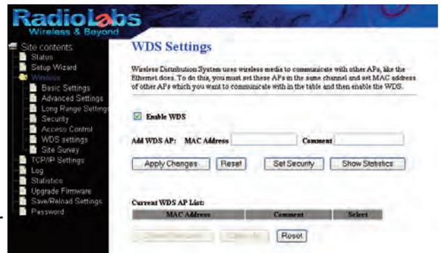
The O2Point Access Point and O2Link Router are now linked by a wireless bridge. Open your browser and enter the O2Link's IP address in the address bar (192.168.1.1) You now should be able to access the Web-Based Configuration Utility of the O2Link's
